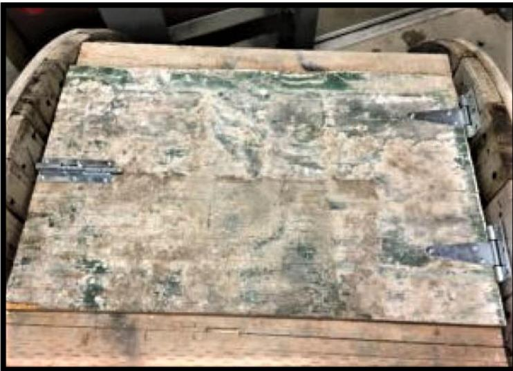
**STEP 3.** Attach the hinges, making sure to leave room for the hinges to swing and bolt to the door. Screw the backs of the hinges to the spool. Test the door a few times to ensure the hinges are secured and that the door opens and closes freely.
