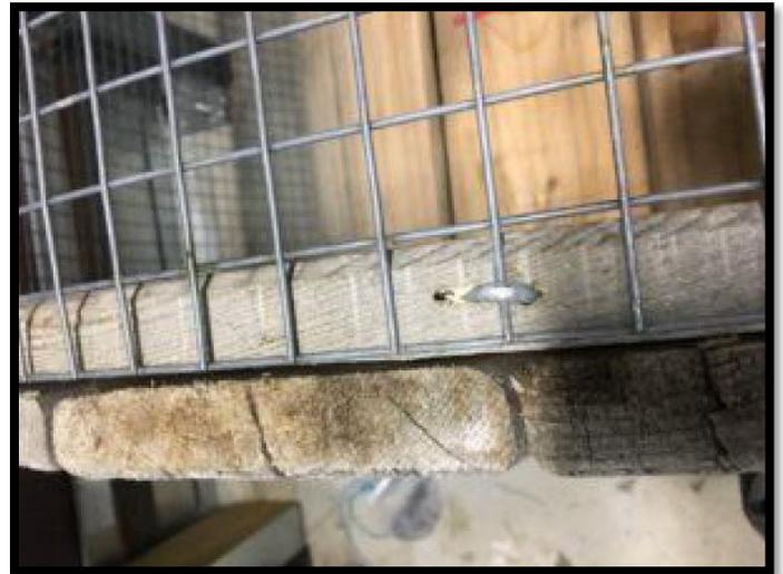
**STEP 6.** After one side is complete, repeat step 5 on the other side of the spool. Check to ensure that the trap door still has enough clearance to open and close easily. If it doesn't, back the pieces of plywood up a bit until it does. It should look similar to the pictures above.
